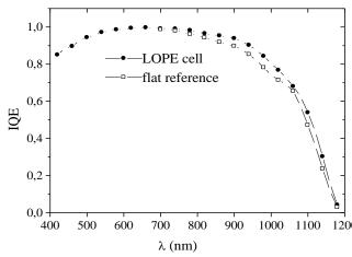
**Fig. 8**: IQE of a LOPE cell and a flat reference (because of technical problems the reference could not be measured over the whole range)
