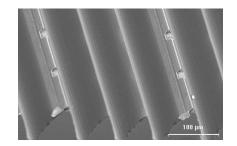
**Fig. 3:** SEM picture of local point contacts on the Vgroove tops of a LOPE cell. The fingers, evaporated under a shallow angle, which are interconnecting the single point contacts, are visible at the V-groove tips (V-groove sequence 3, see text).
