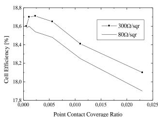
Fig. 5: Optimisation of local point contact distances and comparison of two different shallow emitters ( $L_D=200\mu m$ , full BSF).
