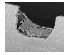
Fig. 4: SEM picture of a single local point contact, which was metallized using the shallow angle evaporation. The width of the point contact openings is approximately  $15\mu m$ .
