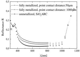
**Fig. 6:** Hemispherical reflectance R of a LOPE solar cell with different point contact distances compared to an unmetallized LOPE cell. All LOPE cells have got an anti-reflection coating, ARC, of SiO<sub>2</sub> and full Al BSF.
