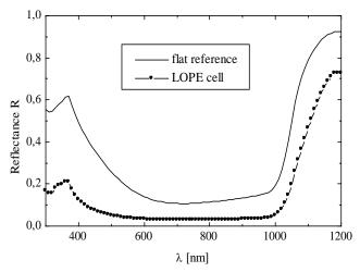
**Fig. 7:** Hemispherical reflectance R of a LOPE solar cell in comparison to a flat reference cell with the same single layer ARC and local BSF.
