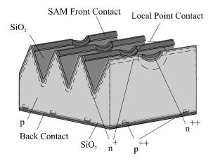
**Fig. 1** Schematic representation of LOPE solar cell structure with a local Al BSF.
