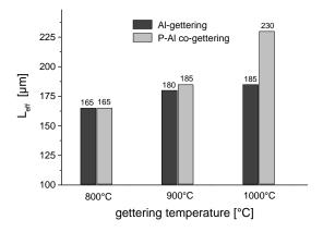
**Figure 2:** Effective diffusion lengths  $L_{eff}$  obtained from a spectral analysis of the IQE in the infrared of Al-gettered (Process A) and P-Al co-gettered (Process B) cells for different gettering temperatures. Given are average values of four cells.
