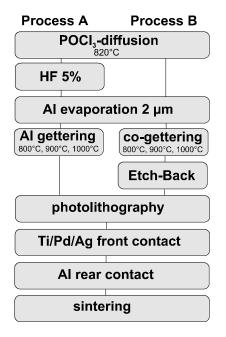
**Figure 1**: Solar cell process for Al-gettering (Process A) and P-Al co-gettering (Process B).
