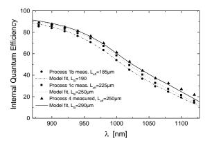
**Figure 4:** Model data (lines) calculated with PC1D and measured data (points) for best cells of Process 1b, 1c and 4.  $L_{eff}$  was obtained from a spectral analysis of the measured curve,  $L_B$  was used in PC1D for the model calculation.
