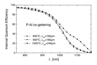
Figure 3: Internal Quantum Efficiency IQE of P-Al cogettered cells at different gettering temperatures.
