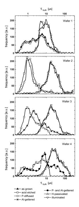
**Figure 4**: Histograms of bulk lifetime mappings performed on different wafers according to the schematic drawing in Fig. 1.
