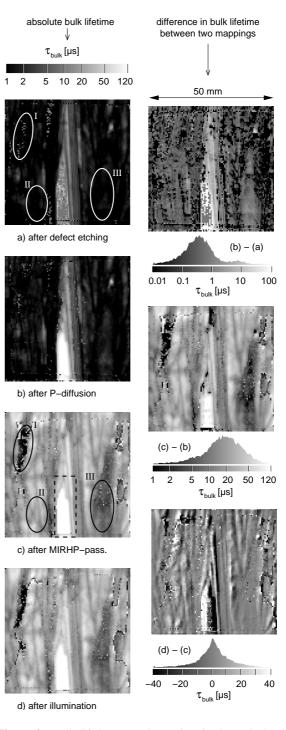
**Figure 2**: Bulk lifetime mappings of wafer 2 as obtained after appropriate combination of various measurements that lead to reliable high and low lifetime values. Left column shows the bulk lifetimes measured after different processing steps with all mappings scaled in the same way. Differences between two steps are illustrated by the right column.
