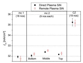
Fig. 2 Mean values and deviation of short circuit density  $J_{sc}$  of solar cells with direct/remote PECVD SiN.
