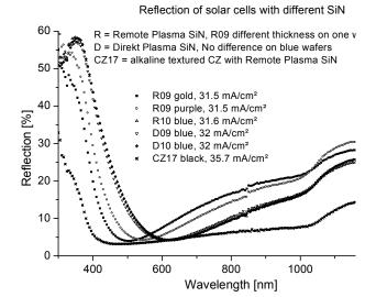
Fig. 5. Reflection of 4 mc and 1 alkaline textured CZ solar cell. Despite the fact that on cell R09 with remote plasma SiN the layer thickness is too thin and the appearance varies from gold to purple there is only a moderate loss in  $J_{SC}$ .
