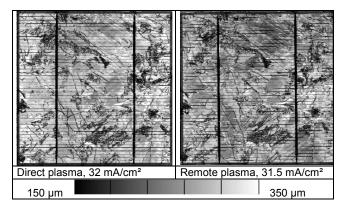
Fig. 6. L<sub>eff</sub> mapping of 2 neighbouring wafers with direct/remote PECVD SiN. LBIC mappings with 833, 910 and 980 nm wavelength were used to calculate  $L_{eff}$ .
