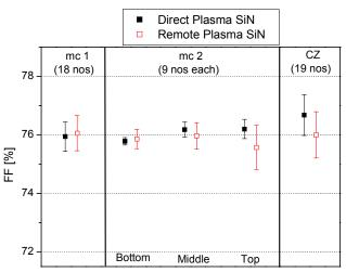
Fig. 3 Mean values and deviation of fill factor FF of solar cells with direct/remote PECVD SiN. No significant difference can be seen.
