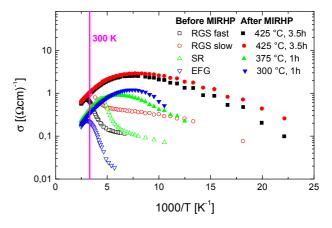
Fig. 3: Conductivity  $\sigma$  before and after MIRHP passivation in ribbon silicon samples originating from the same wafers respectively.
