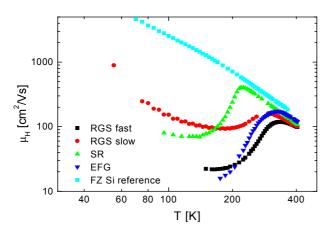
Fig. 1: Hall mobilities of as grown ribbon silicon compared to a monocrystalline reference.
