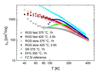
Fig. 2: Hall mobilities of MIRHP passivated ribbon silicon compared to a mono Si reference.
