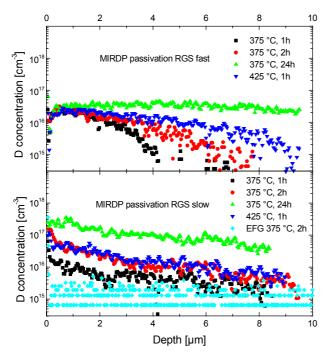
Fig. 4: D concentration profiles determined by SIMS measurements for RGS fast (high [O<sub>i</sub>], top) and RGS slow (less [O<sub>i</sub>], bottom) with EFG as a reference (carried out in collaboration with Bayer AG, Uerdingen, Germany).
