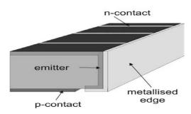
**Fig. 3:** Partial view of a MWA solar cell. The sketch shows the cell edge, where frontside current collecting grid fingers and rear side emitter busbars are connected by a metal strip around the edge.
