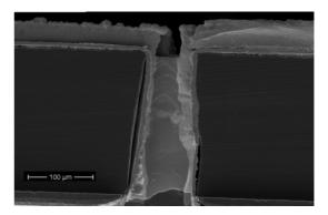
**Fig. 2:** Cross-sectional SEM picture of a hole ( $< 100 \mu m$  dia.) metallised by electroless plating. The hole is perfectly covered with highly conductive copper.
