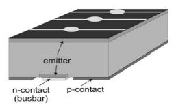
**Fig. 5:** Section of a MWT solar cell. The emitter grid fingers are connected to the rear side busbars via metallised holes.
