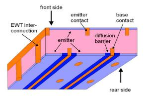
Fig. 7: Schematic view of the bifacial EWT design. The plated metal contacts are orange, the double-sided antireflection coating is light blue and the diffusion barrier is dark blue.
