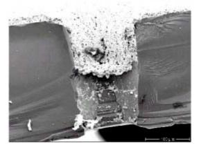
**Fig. 1:** Cross-sectional SEM-picture of a hole (100  $\mu$ m dia.) metallised by a screen printing paste. The paste was applied from the top. The designated front side of the solar cell is at the bottom of the image. The hole was initially completely filled, but during firing the screen printing paste shrunk by about 50%.
