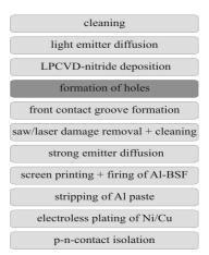
**Fig. 4:** Processing scheme for MWT solar cells based on the buried contact method. The only additional processing step is the formation of a rather small number of holes.
