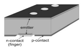
Fig. 6: Section of an EWT solar cell. The frontside emitter is connected to the rear side grid fingers and busbars via a number of holes.
