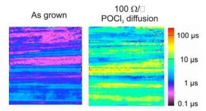
**Figure 4:** Lifetime map of as grown wafer on the left. Improvement after 100  $\Omega$ /sq POCl<sub>3</sub> diffusion (P-gettering).
