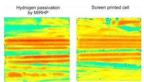
**Figure 9:** Comparison of lifetime maps. Buried contact process (left) to screen printing process (right).
