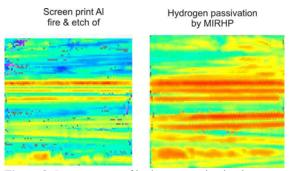
**Figure 8:** Improvement of hydrogen passivation by MIRHP.
