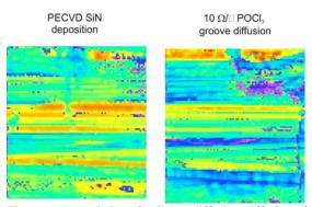
Figure 6: Degradation after heavy diffusion. Effusion of hydrogen.
