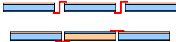
Figure 2: Interconnection of p-type solar cells in a standard module (top) and innovative alternate interconnection of p- and n-type solar cells in a pn-module (bottom).
