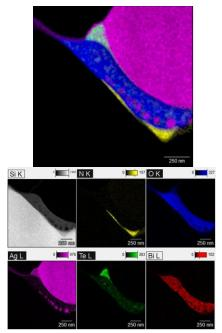
Figure 3: EDX mapped cross section of a Si pyramid
