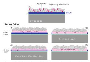
**Figure 1:** Schematic model of contact formation with a PbO-free paste based on TeO<sub>2</sub>.
