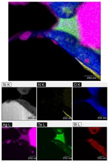
Figure 4: EDX mapped cross-section of a Si pyramid with Ag crystallite at the top, combined on the top, for each element respectively on the bottom.
