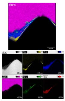
**Figure 2:** EDX mapped cross section of a Si pyramid with Ag crystallite at the top, combined on the top, for each element respectively on the bottom.
