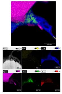
**Figure 5:** EDX mapped cross section of a Si pyramid trough with Ag crystallite at the top, combined on the top, for each element respectively on the bottom.
