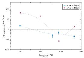
**Figure 6:** Contact resistivity depending on sample peak firing temperature for the same Ag paste on different emitter types.
