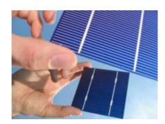
Figure 1. The boron BSF bifacial solar cell. The back side can be seen in the mirror and looks similar to front side
