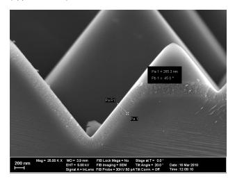
Figure 4 SEM image of a 265 nm layer of porous silicon on a random pyramid textured Cz-Si wafer.
