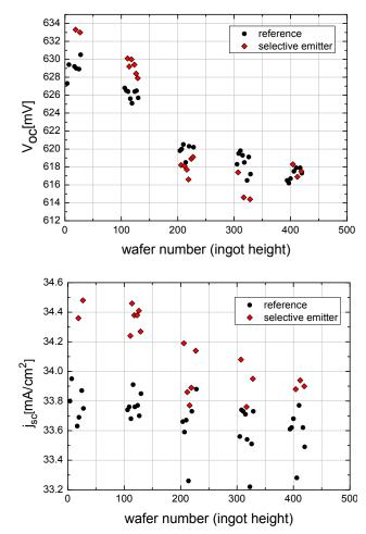
Figure 10  $V_{OC}$  (top) and  $j_{SC}$  (bottom) distribution vs. ingot height of a 6" UMG mc-Si ingot. The best selective emitter solar cell resulted in an efficiency of 16.8 %.
