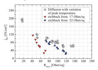
Figure 3 Comparison of  $j_{0E}$  from directly diffused QSSPC samples and emitters etched back from 17 and 52  $\Omega/\Box$ .
