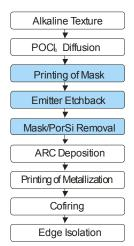
Figure 1 Processing sequence for the production of an etchback selective emitter solar cell. The additional steps to the standard screen-printing process are marked in blue.
