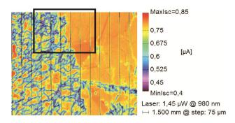
Figure 12 LBIC map of a part of a selective emitter mc-Si solar cell from the top region of the ingot at 980 nm wavelength. The rectangle indicates the area also measured at 405 nm (see Fig. 13).
