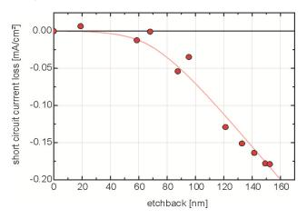
Figure 6  $j_{sc}$  loss vs. etchback depth calculated from measured reflectance data using a typical random pyramid textured selective emitter solar cell IQE. The loss for an etchback of less than 90 nm can be estimated to < 0.05 mA/cm<sup>2</sup>. The red line is a guide to the eye.
