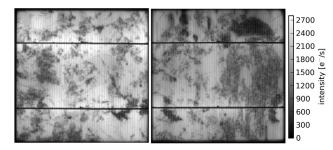
Figure 9 Electroluminescence images of selective emitter solar cells from solar grade mc silicon with a low (left) and high (right) density of grain boundaries.
