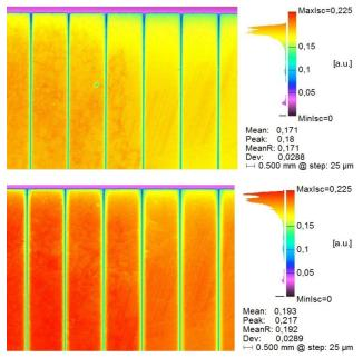
Figure 13 LBIC maps of neighboring mc-Si solar cells from the top region of the ingot. Measurements were taken at 405 nm wavelength from the rectangle marked in Fig. 12.
