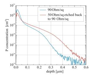
Figure 2 SIMS profiles of a 90  $\Omega/\Box$  direct diffusion and a 50 Ohm/sq diffusion etched back to 90  $\Omega/\Box$ .
