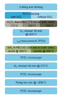
**Figure 2:** Process flow of 1  $\Omega$ cm p-type FZ lifetime samples. For some samples the chemical oxide was removed after the RCA cleaning. Passivation was carried out by Al<sub>2</sub>O<sub>3</sub> deposited at three different temperatures (170°C, 200°C and 300°C), subsequently, some samples were annealed before the first  $\tau_{eff}$  measurement. The SiN<sub>x</sub>:H capping layer of ~120 nm was deposited using a direct PECVD at 300°C or a remote PECVD at 400°C.
