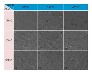
**Figure 6:** SEM images of the surface of  $Al_2O_3/SiN_x$ :H stacks after SiN<sub>x</sub>:H deposition. The 7.5 nm thick  $Al_2O_3$  layer was deposited by plasma-assisted ALD at three different temperatures 170°C, 200°C, and 300°C (displayed in the rows), and the ~30 nm thick SiN<sub>x</sub>:H capping layer coated using direct PECVD also at three different temperatures 300°C, 350°C, and 400°C (shown in the columns).
