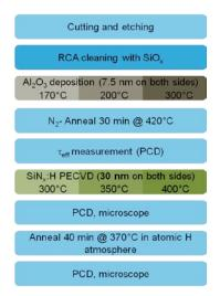
**Figure 1:** Process flow of 1  $\Omega$ cm p-type FZ lifetime samples. The chemical oxide was not removed after the last step of the RCA cleaning. Passivation was performed by Al<sub>2</sub>O<sub>3</sub> deposited at three different temperatures (170°C, 200°C and 300°C). The SiN<sub>x</sub>:H capping layer of ~30 nm was deposited using a direct PECVD at three different temperatures (300°C, 350°C and 400°C) or a remote PECVD at 400°C.
