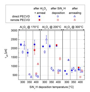
**Figure 3:** Effective minority carrier lifetime  $\tau_{eff}$  dependant on Al<sub>2</sub>O<sub>3</sub> and SiN<sub>x</sub>:H (direct and remote PECVD) deposition temperature. The SiN<sub>x</sub>:H layer thickness is ~30 nm. Measurements were carried out after the Al<sub>2</sub>O<sub>3</sub> post deposition anneal at ~420°C for 30 min (square), after SiN<sub>x</sub>:H deposition (dot) and after an annealing step at 370°C for 40 min (triangle).
