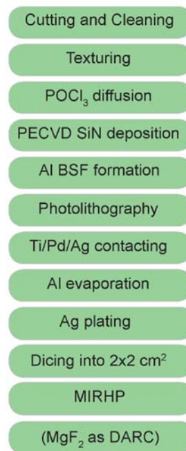
Figure 1: Processing sequence for the applied high efficiency cell process including the plasma texture.
